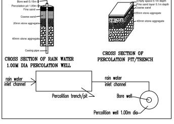
DETAILS OF RAIN WATER HARVESTING STRUCTURES
